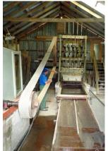
We then toured the gold mining operations from the late 1800s. This belt-driven masher runs on stream water to crush the gold bearing rock.
