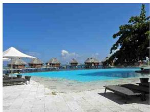
The pool is well engineered to look like it is part of the ocean with no visible far edge. Actually its edge is the skimmer which pours over a board walk set about 3 inches lower so it is not visible. The near edge is gently sloped to look like a beach so you appear to have the beach perspective with the ocean beyond. It was lovely.
